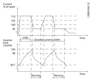
Illustration 3.44 Output Current in Overload Condition
