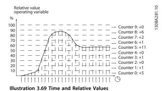
Once a second, the value of the operating variable selected is registered. If a value has been registered to equal 13%, the counter "10% - <20%" is updated with the value "1". If the value stays at 13% for 10s, then "10" is added to the counter value.
