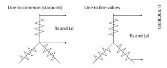
Illustration 3.6 Motor parameters are provided in different formats. Danfoss frequency converters always require the line to common value.
