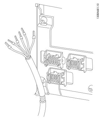
Illustration 1.5 Grounding of Screened/Armoured Control Cables
