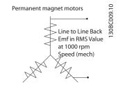
Illustration 3.7 Machine parameter definitions of Back EMF of permanent magnet motors
