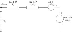
q-axis equivalent circuit
