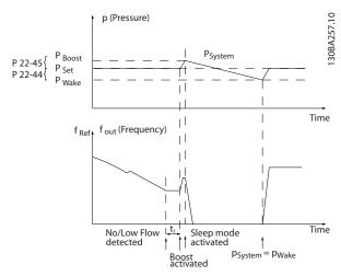
Illustration 3.58 Boost System with Pressure Feedback
