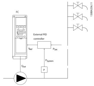
Illustration 3.59 System with Pressure Feedback
