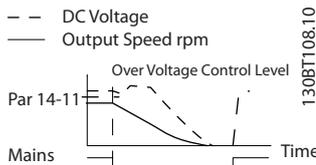
**Illustration 3.34 Controlled Ramp down, longer mains failure.**
