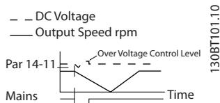
**Illustration 3.33 Controlled Ramp down - short mains failure.**
