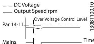
**Illustration 3.35 Kinetic Back-up, short mains failure.**
