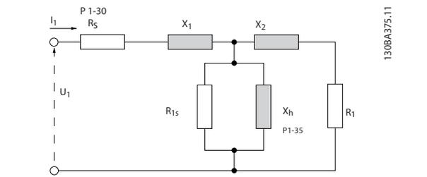
Illustration 3.4 Motor Equivalent Diagram for an Asynchronous Motor
