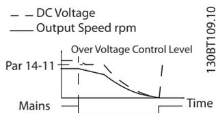
**Illustration 3.36 Kinetic Back-up, longer mains failure.**
