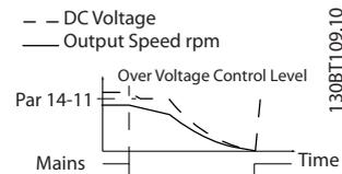
Illustration 3.48 Kinetic Back-up, Longer Mains Failure. The motor is coasted as soon as the energy in the system is too low.
