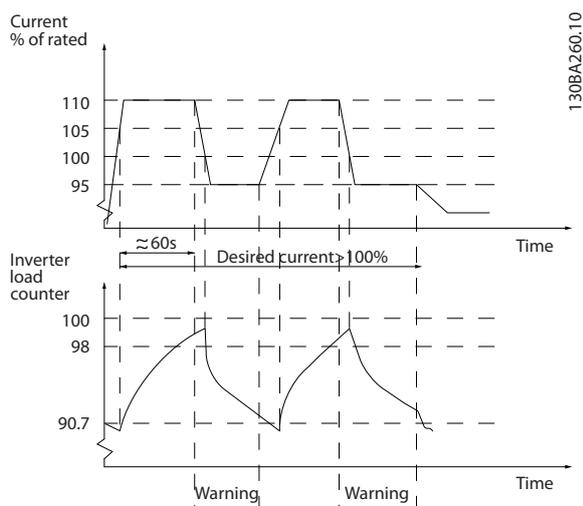
Illustration 3.44 Output Current in Overload Condition
