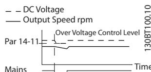
Illustration 3.47 Kinetic Back-up, Short Mains Failure. Ride through as long as the energy in the system allows for it.
