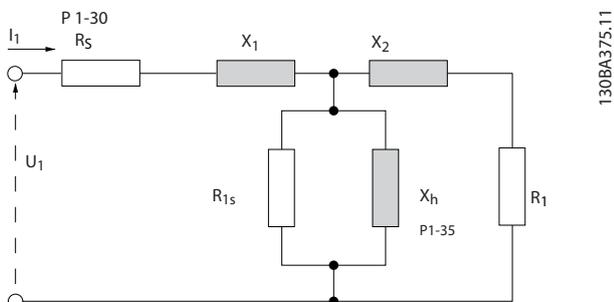
Illustration 3.4 Motor Equivalent Diagram for an Asynchronous Motor
