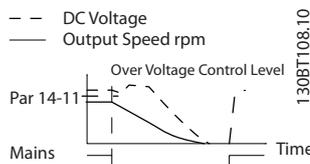
Illustration 3.46 Controlled Ramp Down, Longer Mains Failure. Ramping down as long as the energy in the system allows for it, then the motor is coasted.
