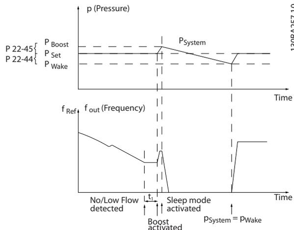
**Illustration 3.58 Boost System with Pressure Feedback**
