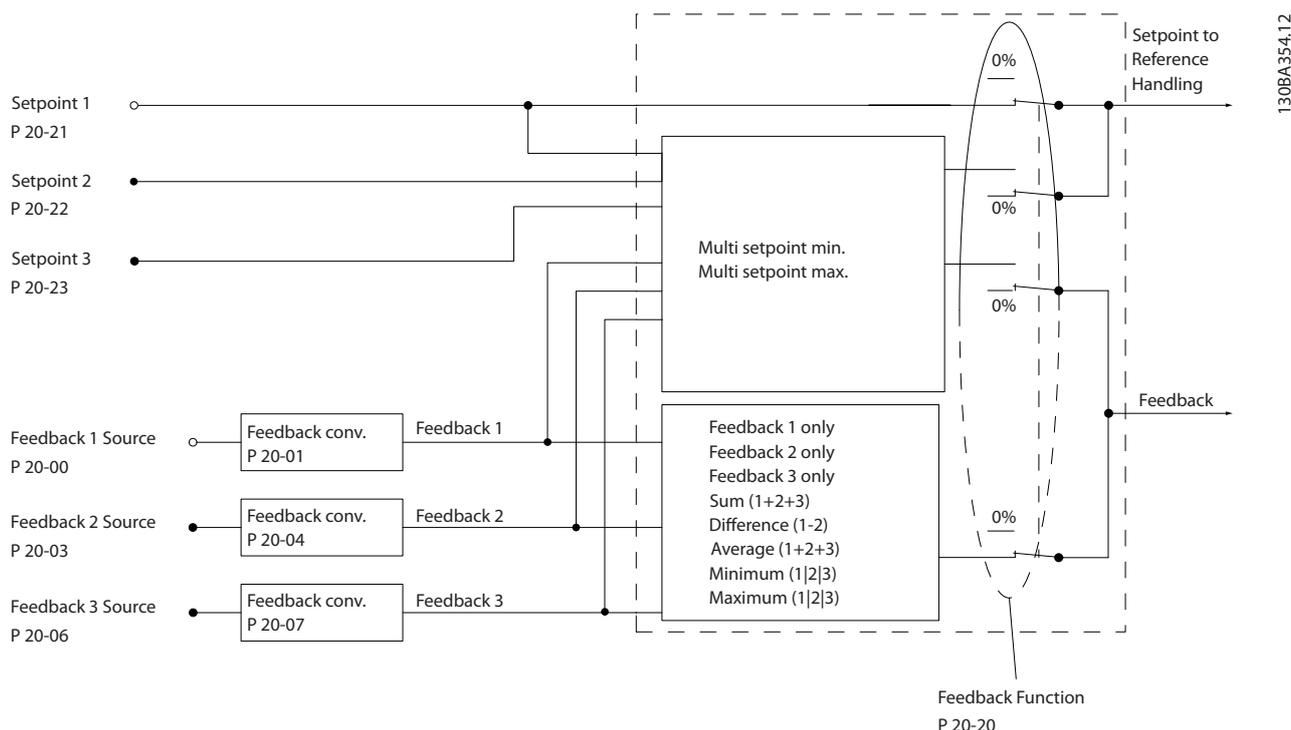
Illustration 3.51 Input Signals in Closed Loop PID Controller
