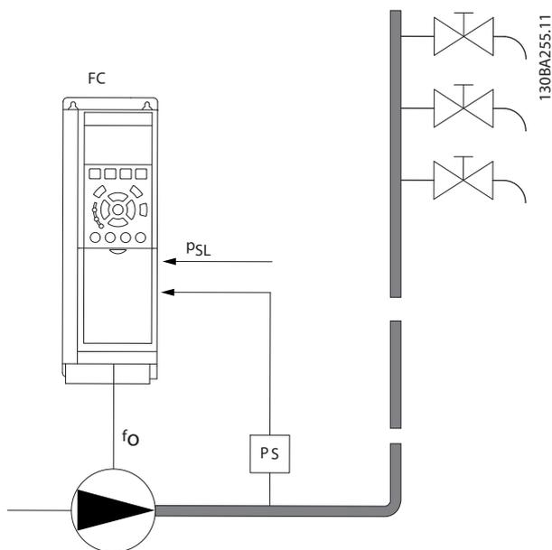
**Illustration 3.57 Legend:** FC=frequency converter; f<sub>o</sub>=frequency out; P<sub>s</sub>=P system; P<sub>SL</sub>=P setpoint
